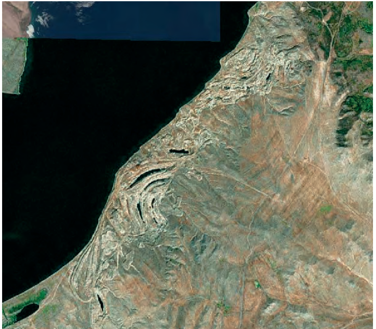
The nature of soil degradation at the Gusinozersk brown coal field: open pits filled with water and waste rock dumps.
