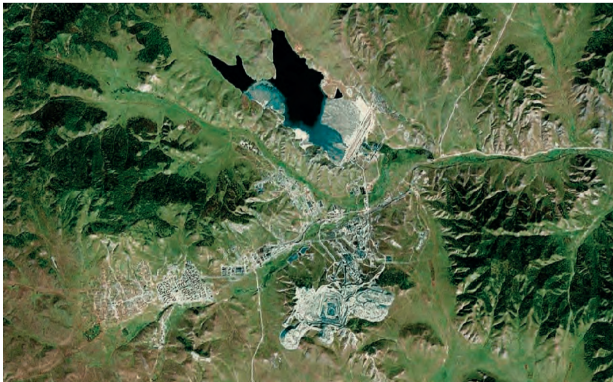
Production and social infrastructure facilities at the copper molybdenum deposit Erdenetiyn Ovoo. There is a tailings pond in the northern part of the photo. The open pit is shown in the southern part, while production and residential zones – in the southwest.
