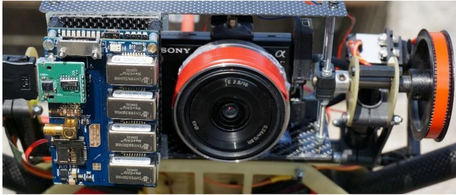
Fig. 2. Sensor mount for direct georeferencing
