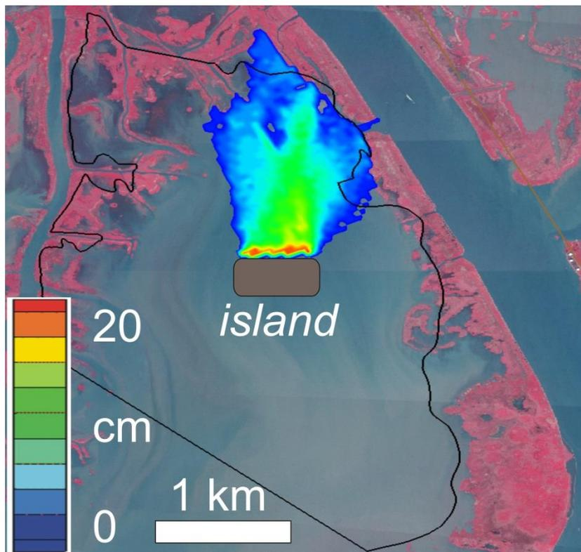
Fig. 3. False-color satellite image of West Bay, with schematic of dredge-spoil island location, and plot of wave-height reduction produced by island construction. Bar scale of wave-height change in cm
