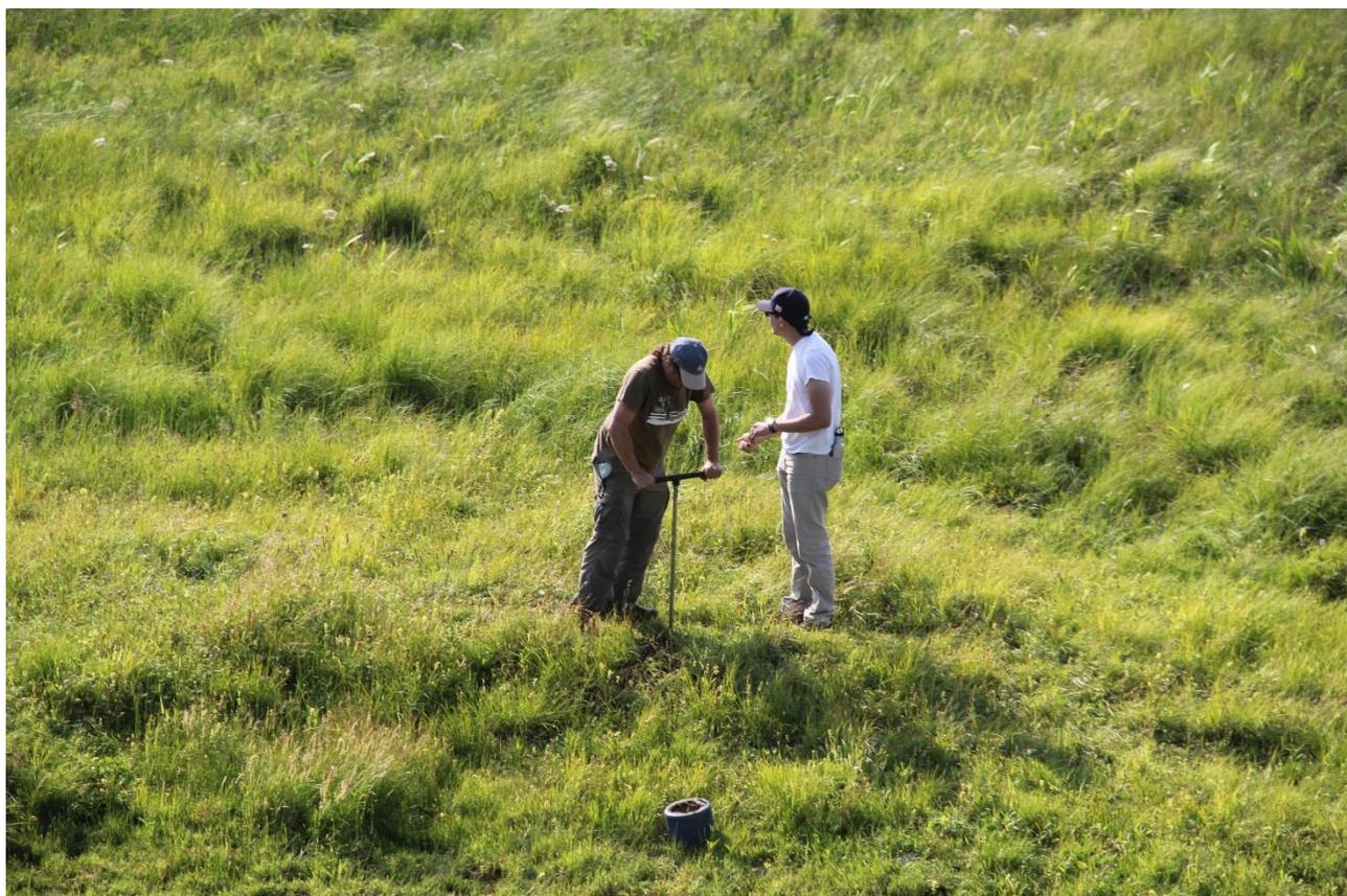
Soil sampling with the soil tube
