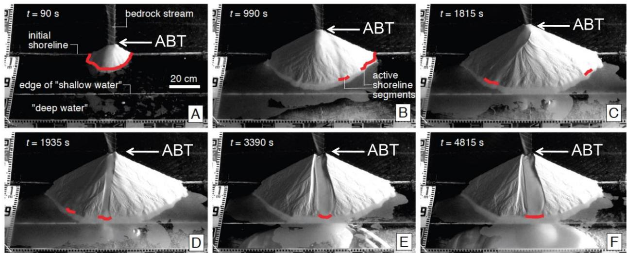
Fig. 1. Sequential photo images of an experimental run of the "fixed-boundary" series. Note that soon after the delta toe reached the submerged overfall, distributary channels evolved to a single large channel that was stabilized in the axial part of the delta plain. Red lines indicate active shoreline segments. ABT = alluvial basement transition
