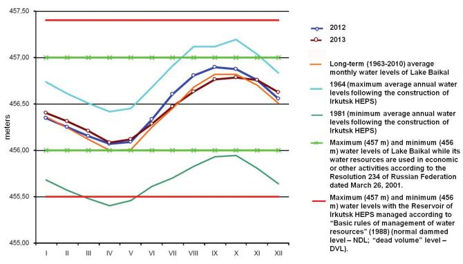
Pic. 1.5.3 Average monthly water levels of Lake Baikal in 2012 and 2013 compared with the years of the highest (1964) and lowest (1981) levels and long-term values.
