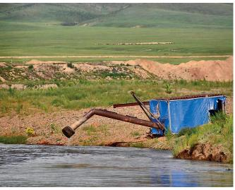
Pic. 4.2.11 Tail dumps and wastewater discharge point of a goldmining enterprise (Zamaar soum, Tuv aimag)
